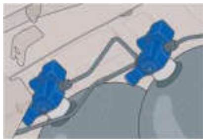
Electromagnetic shut-off valves on the gas tanks
